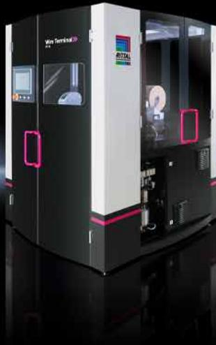
The new, compact Wire Terminal WT fully automated wire processing machines produce up to 36 different wires in cross-sections ranging from 0.5 mm<sup>2</sup> to 2.5 mm<sup>2</sup> (AWG 20 - 14) automatically, with zero manual intervention.
