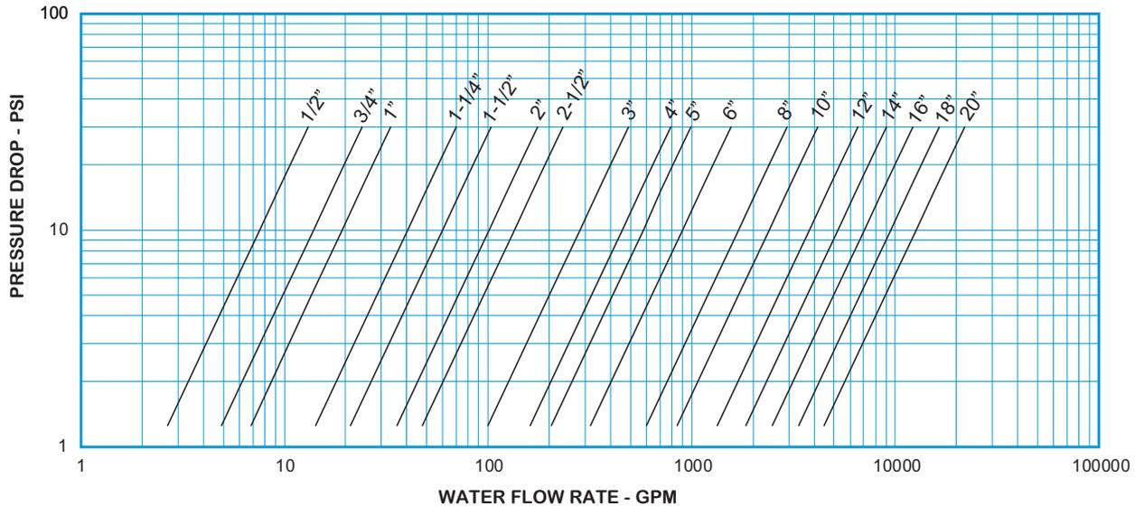
**Note:** All flow curves and Cv values presume the valves are fully open with 1/2 PSI cracking pressure springs. Consult the factory for more information.
