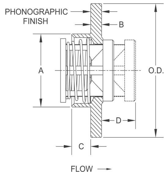
❶ Check “A” dimension for clearance with pipe ID. Generally “A” dimension is designed for use in schedule 40 pipe for class 150 & 300 valves (F1). Order class 600 (F6) valves for schedule 80 pipe.
